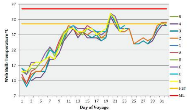
Figure F.4. Comparison of mid-morning wet bulb temperatures by deck (see legend) and day of voyage, and heat stress threshold (HST; —) and mortality limit (ML; —) (source: Mortality Investigation Report 46, Qatar and the United Arab Emirates, September 2013.)
